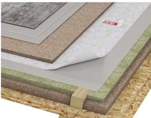
During 2015 Eterno Ivica has designed the underlay TXT, manufactured using fully recycled materials and recyclable, to reduce impact noise on floors. TXT has been patented. Under screed resilient underlay ECOTEX LIGHT TXT 7 mm thick made from cotton waste of white colored fabrics, obtained from a sanitized and sterilized mixture of filaments of cotton, linen and wool, maintained in plates of dimensions 1.20 m x 2.00 m by means of adhesive polypropylene.
